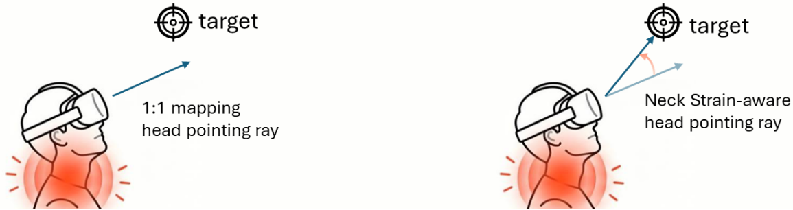
Figure 1: Strain-aware head pointing. Left: 1:1 mapping head pointing cannot reach the target, and neck strain occurred. Right: Neck strain drives the cursor and amplifies the pointing ray angle, enabling target acquisition.
